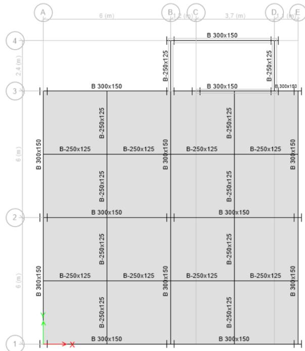
Figure 2. Structure typical floor plan
